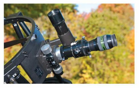
▲ The Stargate comes with a 9×50 straight-through finder and a 2-inch, two-speed focuser with extension tubes/adapters for 2- and 1¼-inch eyepieces. As explained in the accompanying text, the author typically observed with the Tele Vue Paracorr coma corrector pictured here.
